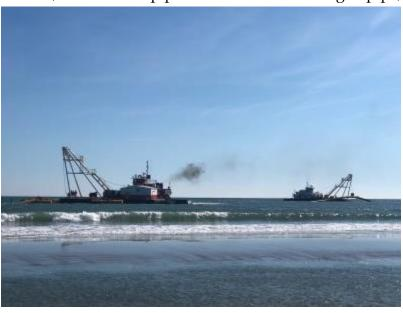
be used as the main transport for sand from the inlet to the Topsail Beach/Surf City line. The dredge *J.S. Chatry* will be working in the inlet. The line connecting the submerged pipe to the beach is located just south of Queens Grant, as nourishment work will move northward from that location at the start of the project. Once the northern stretch is completed, the project will begin to move south. In early
